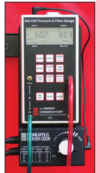
DG-700 Pressure and Flow Gauge with Cruise feature
