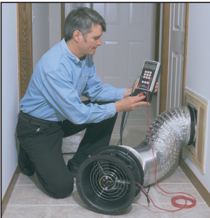
The Minneapolis Duct Blaster® is used to measure the airtightness of duct work.
