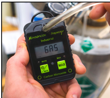
Connect the 50ppm calibration gas.
