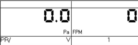
**MODE** To select the **Pressure/Velocity** mode, press the **MODE** button until the selected operating mode shown on the gauge display is **PR/ V**. When first entering this mode, the default air velocity unit on **Channel B** is feet per minute (FPM). **Channel A** always displays pressure readings in Pascals when in the **PR/ V** mode.
