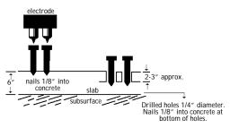
If the meter still indicates green or "dry" the floor is ready for covering. Tests should be made at several points, especially when the slab is thick and air circulation is poor. Tests should only be made in newly drilled holes, since the inside surface of the holes can dry out while the rest of the slab is still wet.
